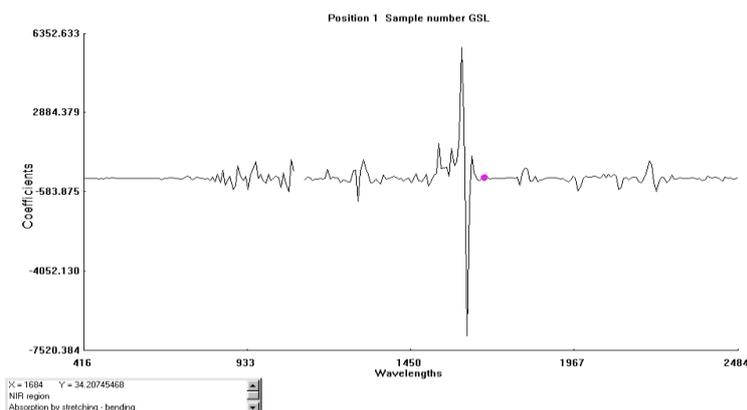
Figure 2. Plot of wavelength correlation with glucosinolate contents (Butkute, 2003b).
